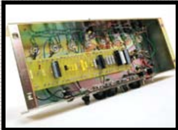
■ Inside the amp chassis, the components are neatly hand-wired onto traditional turret board
